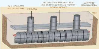
Note: In traffic areas – concrete ceiling is a must. Non-traffic areas – maximum backfill allowed – 25-30cm.
